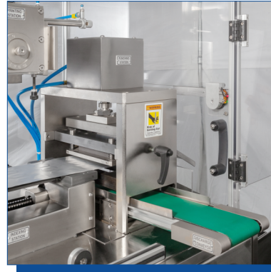
PUNCHING TOOL WITH DISCHARGE CONVEYOR FOR SMOOTH PRODUCT HANDLING
