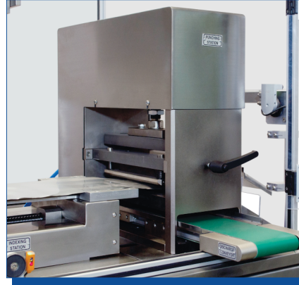
PUNCHING TOOL WITH DISCHARGE CONVEYOR FOR SMOOTH PRODUCT HANDLING
